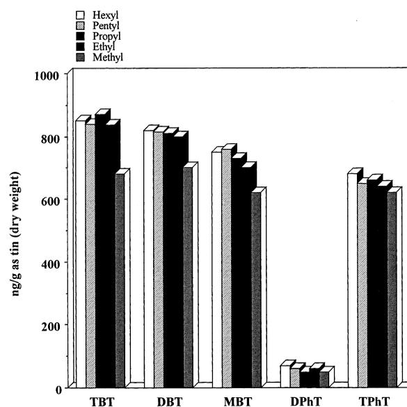
Fig. 2. Comparison between different Grignard reagents in the determination of organotin compounds in mussel tissue (final volume = 1 ml).
